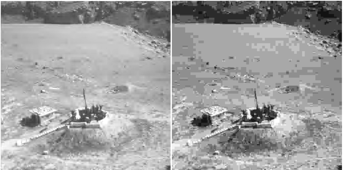
Figure 9, Target Detection and Compression @ 50:1 (0.16 bits/pixel). Left - Combined Fuzzy Mask-based wavelet, Right - JPEG for comparison. The PSNR measurements being 26.91 and 22.69 respectively.
