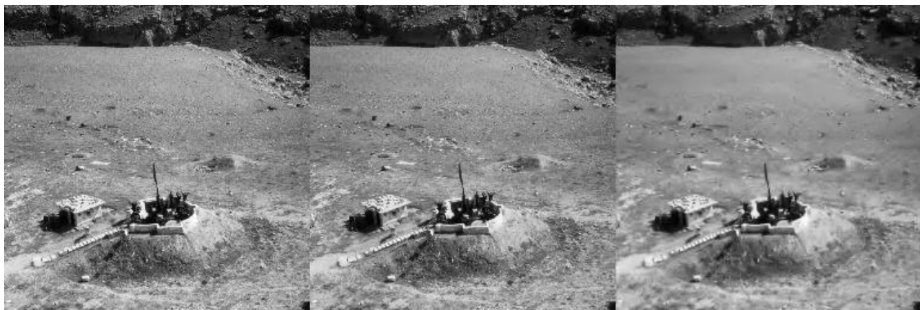
Figure 6, Wavelet reconstruction after removal of 30%, 60% and 95% of weakest coefficients.
