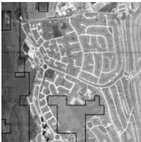
Figure 5. Output from the PBN image segmentation algorithm, showing the segmentation of a reconnaissance image into urban and non-urban regions.
